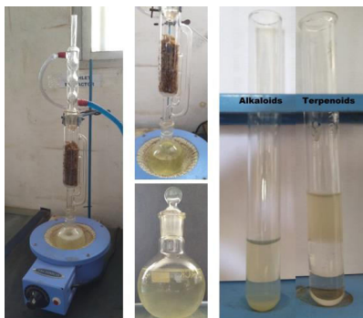
Fig. 1: Extraction of Zoochemicals using Soxhlet method and qualified.
