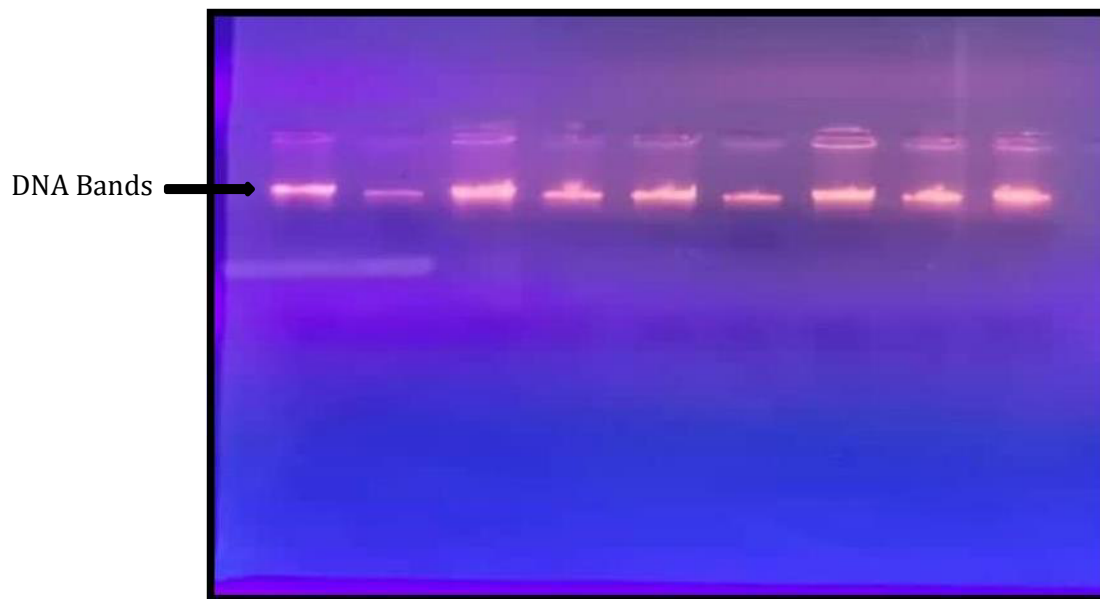
Fig. 1: Electrophoresis of chromosomal DNA bundles extracted from blood samples of alopecia areata patients and healthy subjects and carried over on agarose gel with a concentration of 1% and an electric potential difference of 100 volts/30 min.
