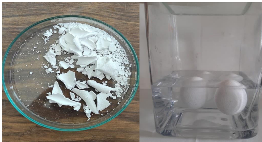
(a) (b) Fig. 4: (a) Calcium oxalate crystals and (b) decalcification of egg shell in 10% HCl.
