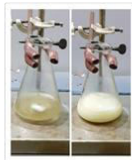
Fig. 2: Synthesis of zinc oxide nanoparticles from extract of Elettaria cardamomum (seed pod).
