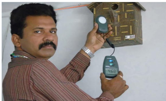
Fig. 1: Measuring light illumination by Lux meter.
