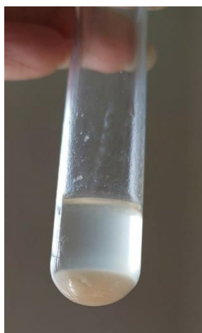
Fig. 3: Glycolipid precipitated at the bottom.
