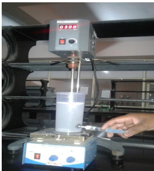
Fig. 1: Photograph showing technique used for fabrication of floating Microsphere.
