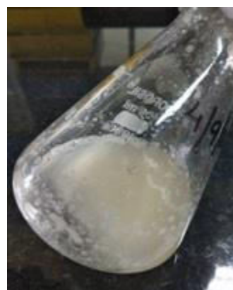
Fig. 3: Filter paper degradation test ( Day 12).
